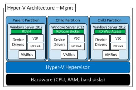
Management role requirements for the base solution are summarized below. Data disks should be used for role-specific application files/ data, logs, IIS web files, etc and should exist in the Management volume on the 4100E array. Please note that the Tier2 volume presented to the file server is designated as a pass-through disk (PTD).
