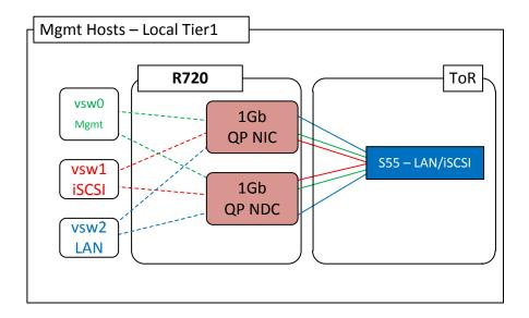
NIC teaming should be configured in the Hyper-V host using Dell drivers to ensure that the proper NICs from differing PCIe devices are bonded. The resulting teamed virtual NIC should then be assigned to the appropriate virtual switch within Hyper-V. VLAN IDs should be specified in all virtual switches used within the Management layer Hyper-V host. All NICs and switch ports should be set to auto negotiate.
